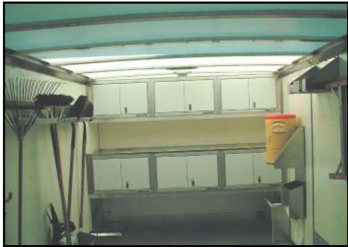
Translucent Roof composite wall lining Extruded Aluminum floor and ATP wall guard standard
